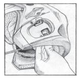
5. Use the provided Allen wrench and screw, and tighten until Sena clamp is secure.
