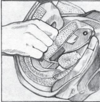
2. On the left side, you will see a red tab. Pull on this tab to remove the EPS plug.
