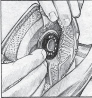
8. Replace the cheekpads, pull the chin straps through the openings the cheekpads, and then secure the 2 snaps at the back of the helmet, making sure the speaker wiring is hidden beneath the padding.
