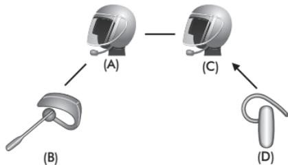
4. Now two SMH10 headsets (A & C) and two non-Sena Bluetooth headsets (B & D) are connected with the four-way Universal Intercom.
