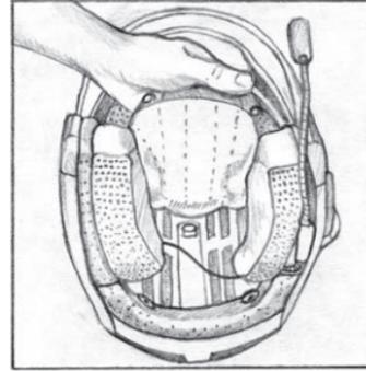
7. Open the Velcro closure on the speaker pockets and place the speakers inside before securely closing again.
