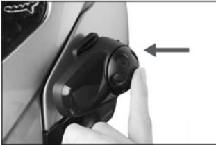
3. To track forward or track back, rotate while pressing the Jog Dial clockwise or counter clockwise.
