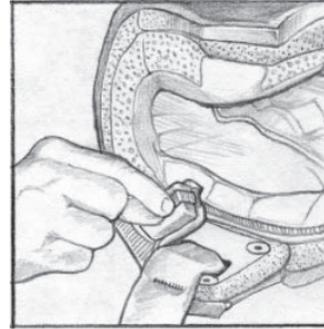
3. Next, remove the trap door on the left side of the helmet.
