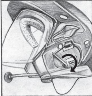
6. Lift up the helmet top padding from the back of the helmet (connected by 2 snaps) and route the speaker wires beneath the padding.
